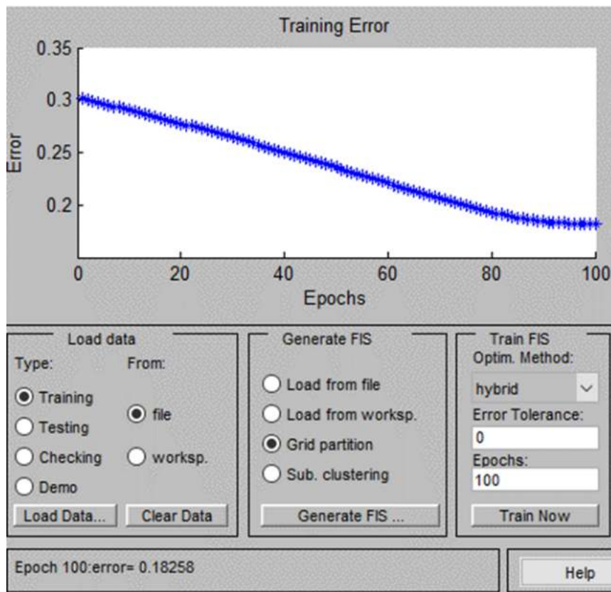
Figure 9: Training data and determination of ANFIS programming tolerance errors
